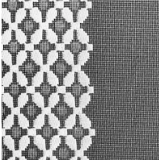
Raschel knit curtain with inlay threads over a marquisette ground, and detail showing the lighter inlay threads held by each knitted pillar, and the heavier inlays held only at their extremities. ( 7 Earnshaw p. 64-5)
