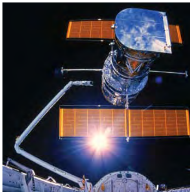
The Hubble Space Telescope being released into orbit by the space shuttle. Image courtesy NASA.
