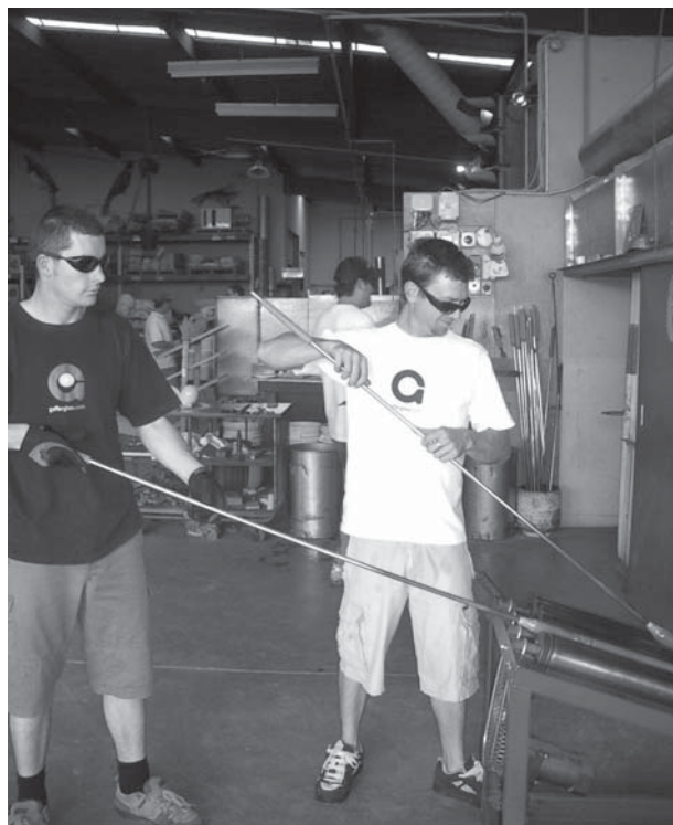
Jim Edmonds and Eddie Neale hand roll rods of coloured glass from hot glass gathered from the furnace, 2006. Photo: John Croucher
