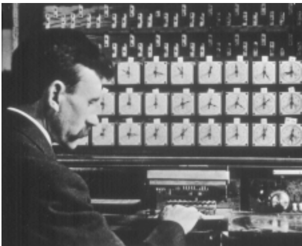
The Hollerith tabulator was developed by Herman Hollerith in 1887 after the 1880 US census, to sort and count census data. Photo: the Hollerith Tabulator, which used punched cards, was also adopted by business and science, Library of Congress.
