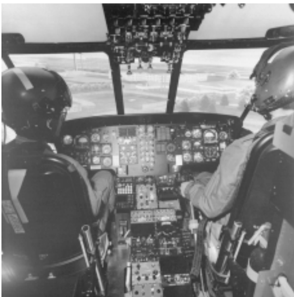
Computers can combine mechanical, functional and aerodynamic data to create a replica of the workings and operations of an aircraft, such as this Sea King simulator. Photo courtesy of Thomson-CSF Pacific Pty Ltd.
