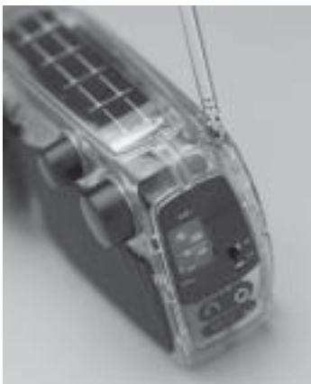
The Freeplay wind-up radio needs no coal-fired electricity. It is powered by either arm muscles or the sun. When you wind the handle it tightens a spring inside the radio that stores enough energy to play for 45 minutes. Photo by Sue Stafford, Powerhouse Museum
