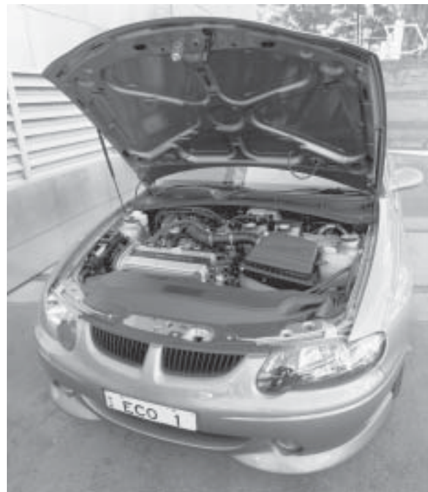
The engine of the ECOMmodore, the first hybrid petrol-electric car to be built in Australia. Lent by Holden Ltd for the exhibition EcoLogic: creating a sustainable future . Photo by Marincio Kojdanovski, Powerhouse Museum
